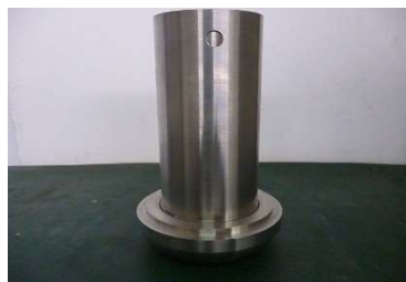
Stand Pipe Pressure Transducer
